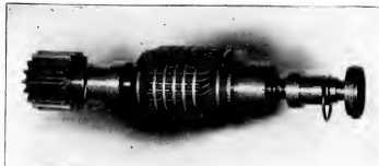
CONSOLIDATED CAR LIGHTING SYSTEM—ARMATURE RING OILERS AND PINION.
